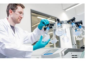
Compact, high-performance tabletop unit for effective lyophilisation of specimens in your everyday lab activities. The condenser temperature of -55 °C enables the drying of aqueous products.
