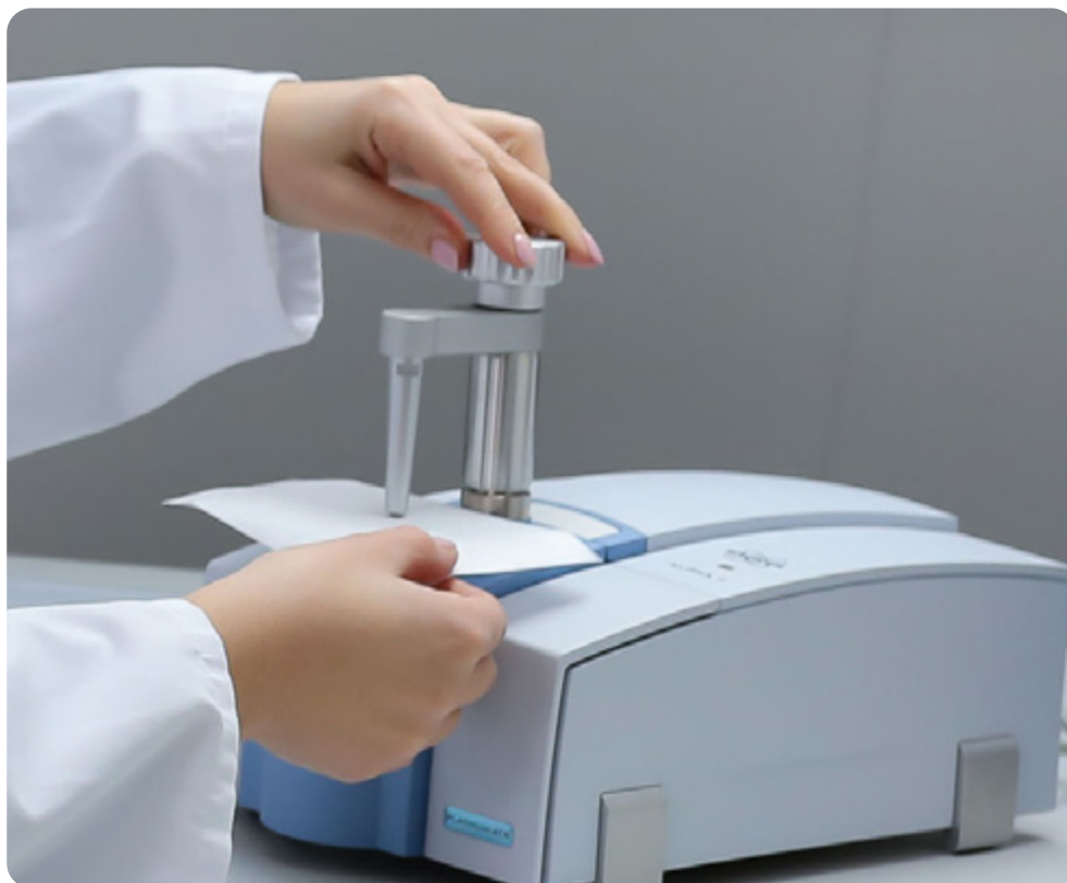
Receiving inspection of membrane with FTIR spectrometer
