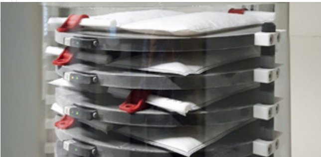
Lyoprotect® Bag DF in use in a laboratory freeze dryer, courtesy of Cilian AG
