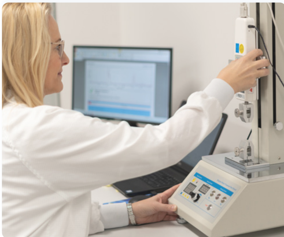
Seam strength test as part of lot release testing
