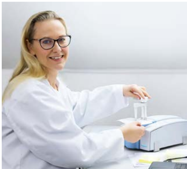
Receiving inspection of membrane with FTIR spectrometer
