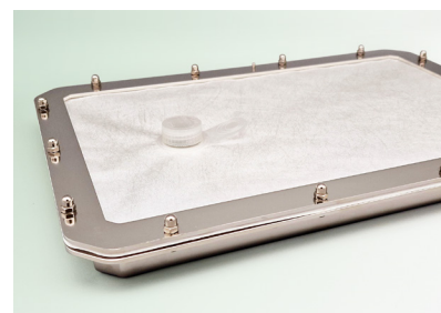
Lyoprotect® Stainless Steel Tray V2740B, membrane with filler assembly
