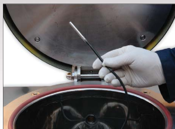
Flexible PT100 Thermoprobe (on request)
